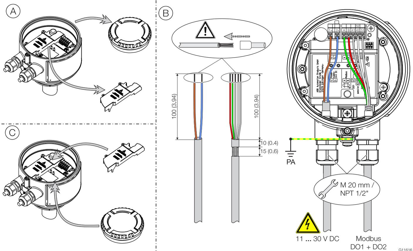
Fig. 26: Connection to the device (example), dimensions in mm (inch)
