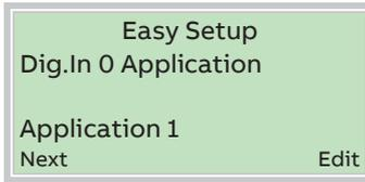
The application is selected if both digital inputs are inactive.
