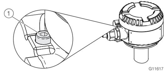
**Fig. 21: Cover safety device (example)**
