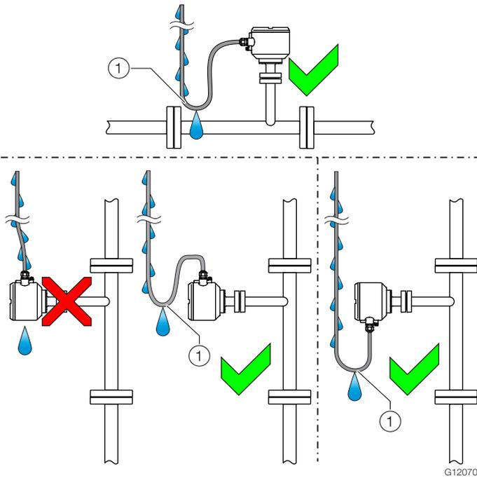
Fig. 22: Laying of the connecting cable
