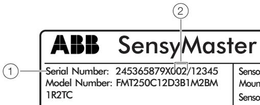
Fig. 28: Modbus address on the name plate (example)
