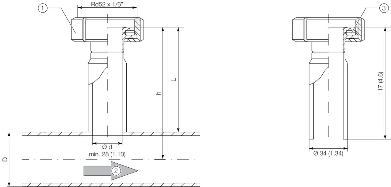
**Fig. 16: Dimensions in mm (inch)****① Union nut ② Flow direction ③ Centering pin**
