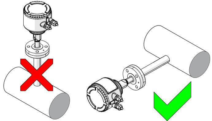
Fig. 7: Mounting position at high ambient temperatures
