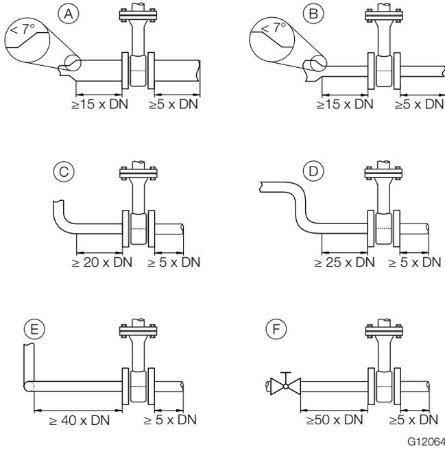
Fig. 6: Inlet and outlet sections
