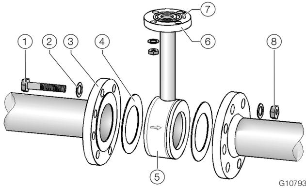
**Fig. 13: Installing a pipe component (example, wafer type design)**
