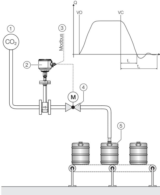
Fig. 32: Filling function FillMass (example CO<sub>2</sub> filling)
