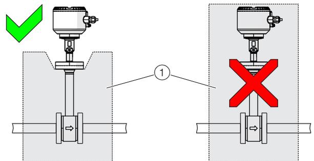
Fig. 8: Insulation of the sensor
