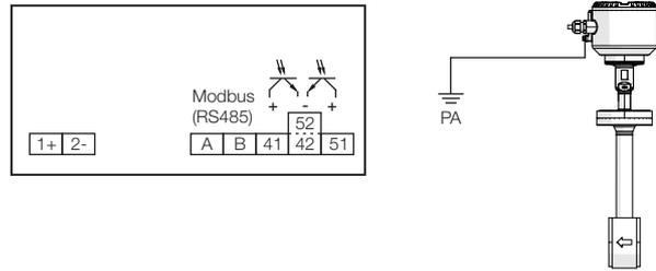
Fig. 23: Electrical connection
