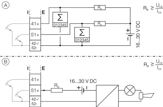
**Fig. 24: Passive digital outputs (I = internal, E = external)**
