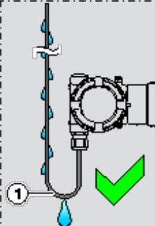
**Figure 13** Typical LWT HART connection
