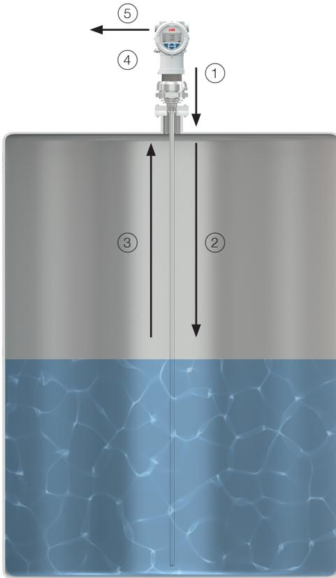
The head sends a very short pulse of microwave energy through the coupler and down the probe ①. That pulse travels along the length of the probe ② and, when it encounters the product surface, some of the energy is reflected and travels back towards the coupler ③. When the reflected energy reaches the coupler, it is sensed by the electronics ④. By measuring the time elapsed between the initial pulse and the reflected one, the electronics can calculate the product level ⑤.
