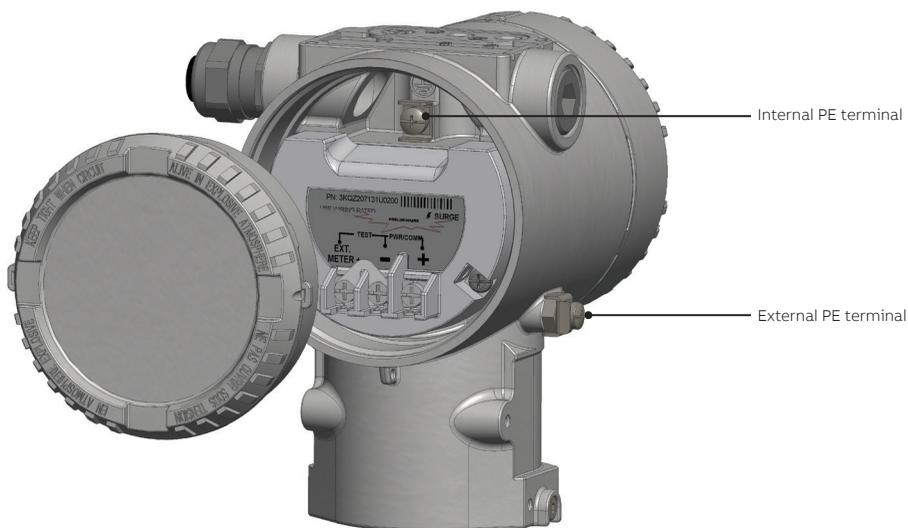
**If using the external PE terminal, you must** connect the grounding wire to the monitored vessel.
