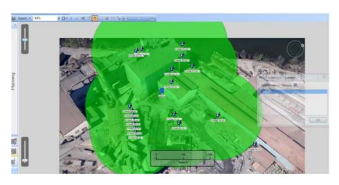
and its meshing provides for a strong network with only a few routers needed, which help make the network even stronger. Depending on the application, we also saved 50-80% with *Wireless* HART compared to the costs of a wired system."
